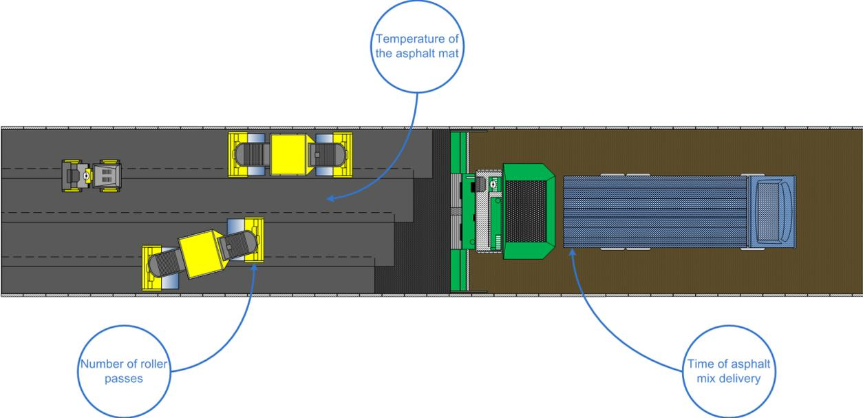
Figure 1. Implicit variables of the asphalt compaction process
