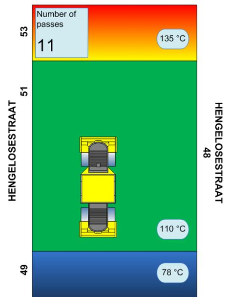
Figure 7. Draft of the data representation for roller operator
