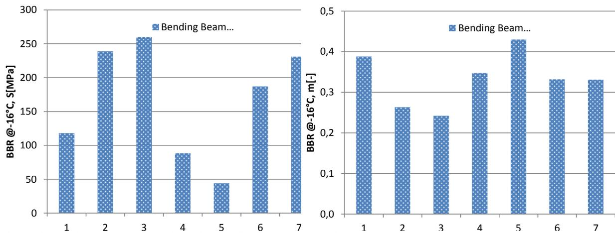
Fig.7 Overview: BBR results after RTFOT+PAV aging
