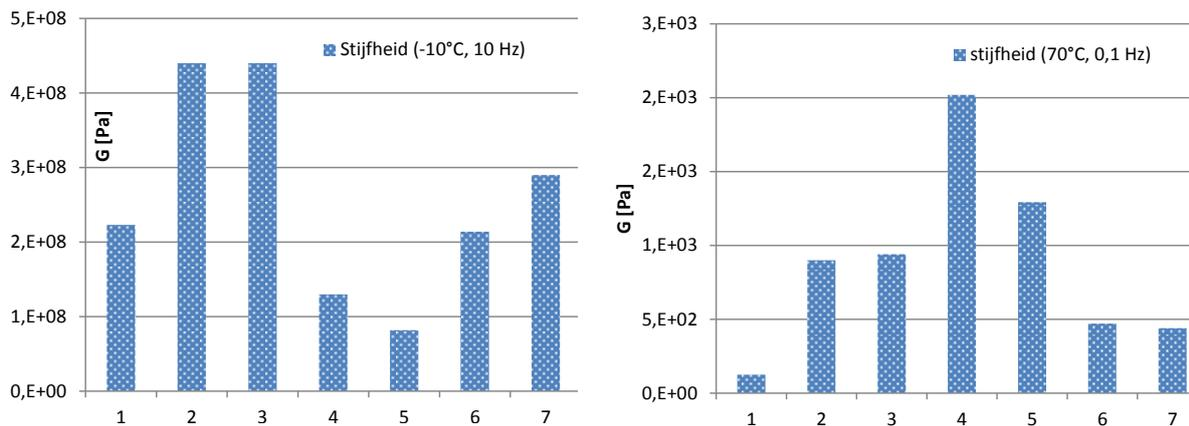
Fig.6 Stiffness properties at low and high temperatures; after RTFOT+PAV aging
