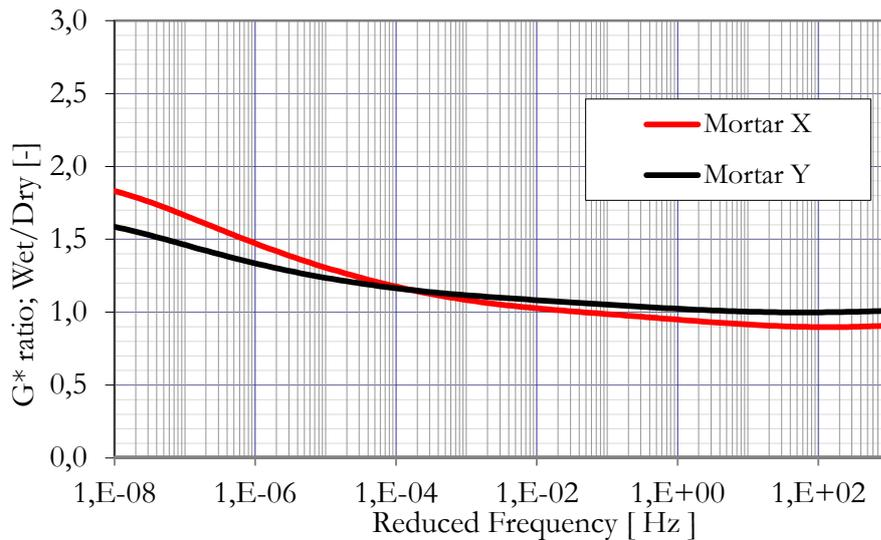
Fig.8 Effects of water on mortar response.
