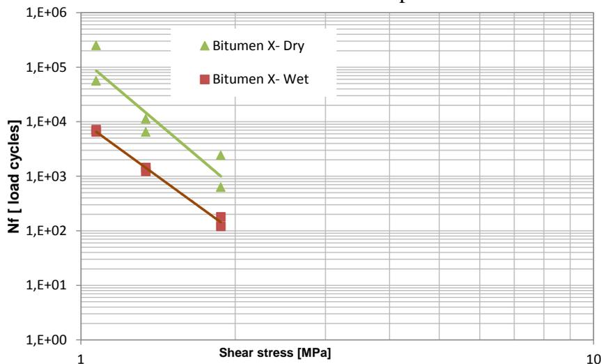
Fig. 9 Effect of moisture on adhesion performance
