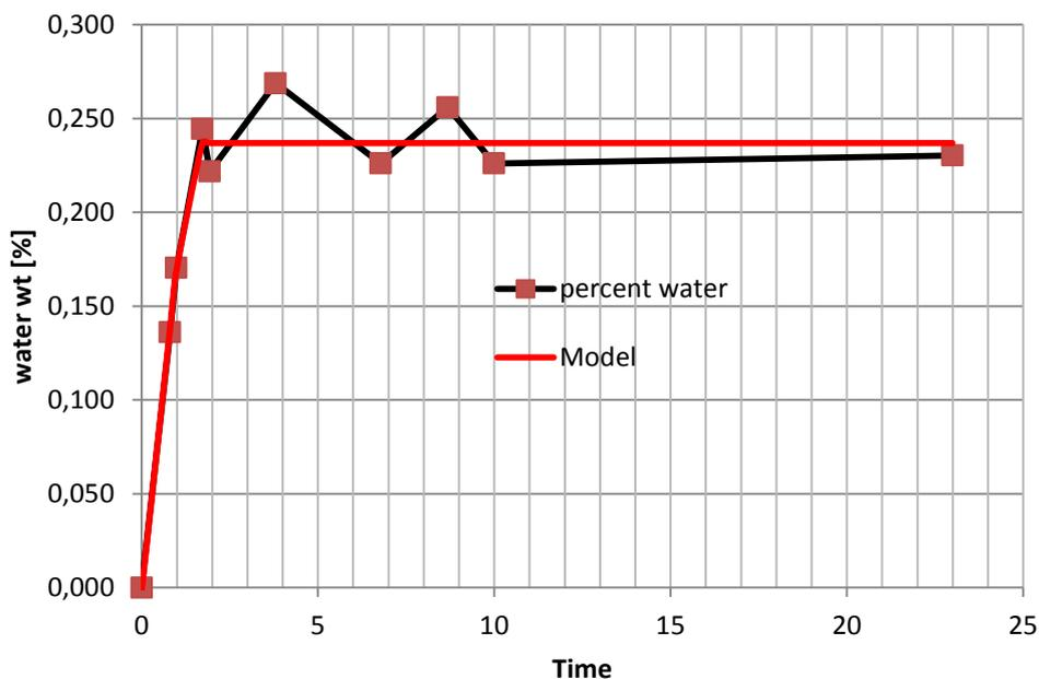
Fig. 3: Illustration: moisture absorption rate for aggregate
