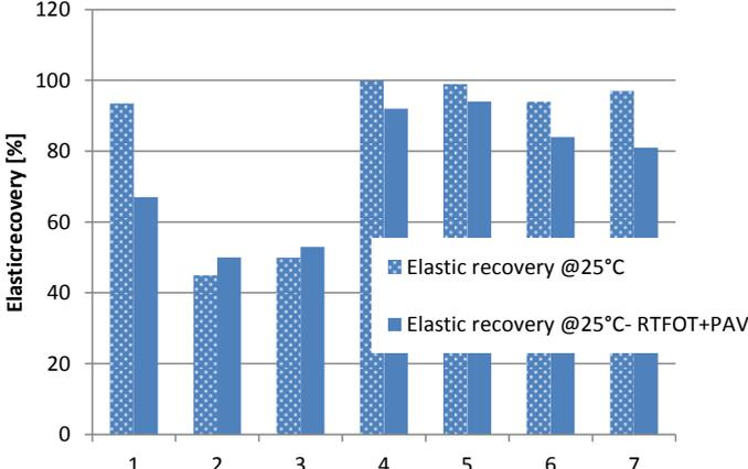
Fig.5 Elastic recovery before and after RTFOT+PAV ageing
