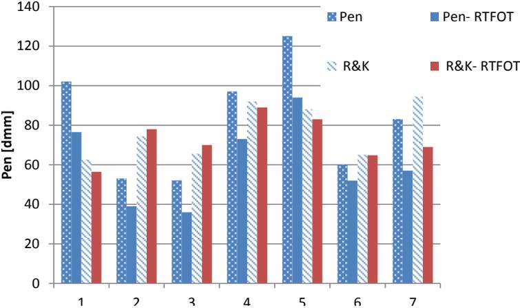
Fig.4 Penetration and Ring&Ball test results for various bitumen before and after RTFOT
