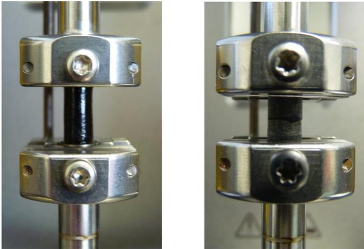
Fig. 2: DSR setups for mortar and stone-column tests
