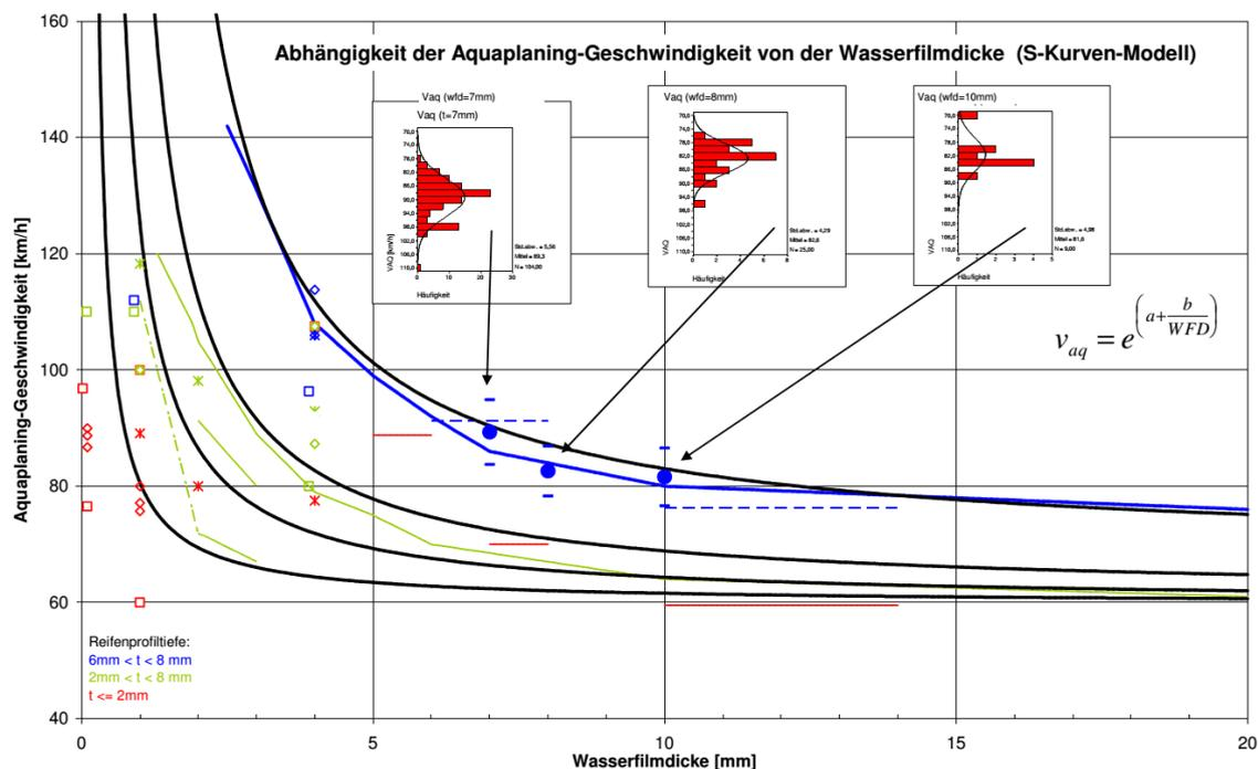
**Figure 3 Hydroplaning speed model for 8, 4, 2 and 1 mm tread depth (black lines), together with experimental data of several authors (colours) and hydroplaning tests on new tyres (frequency curve inserts, summarised in graph as blue ball average and blue dash standard deviation)**
