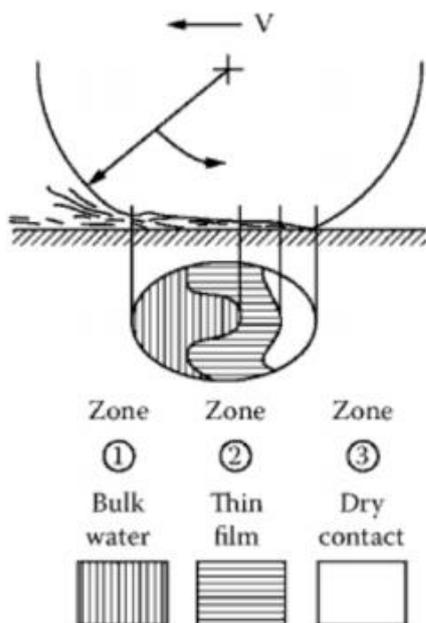
Figure 1 Three-zone concept for tyre-water-pavement interaction [Flintsch et al. 2014]
