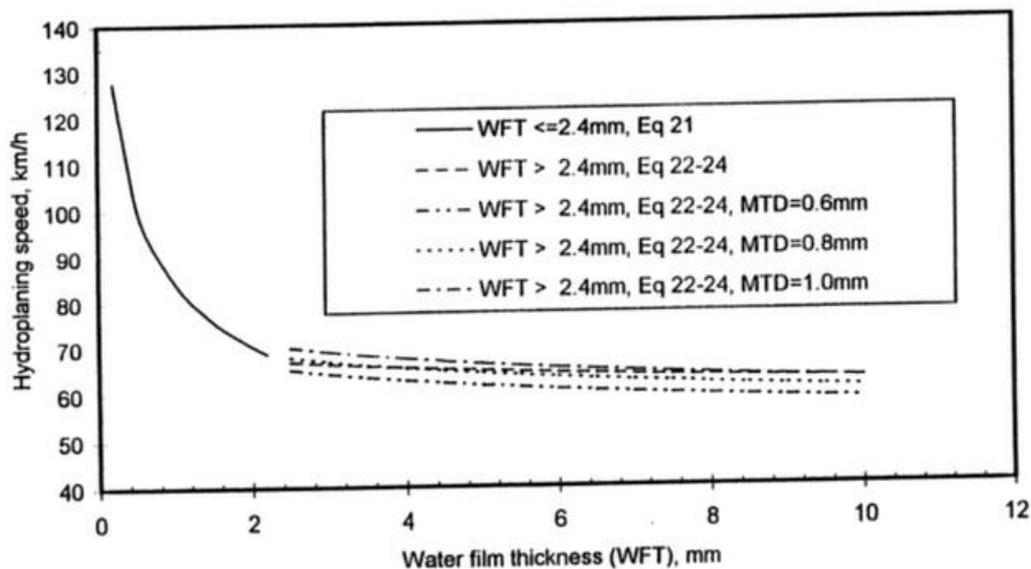
**Figure 2 Hydroplaning speed formula in PAVDRN, (MTD = pavement texture depth) [Anderson et al. (1998)]**
