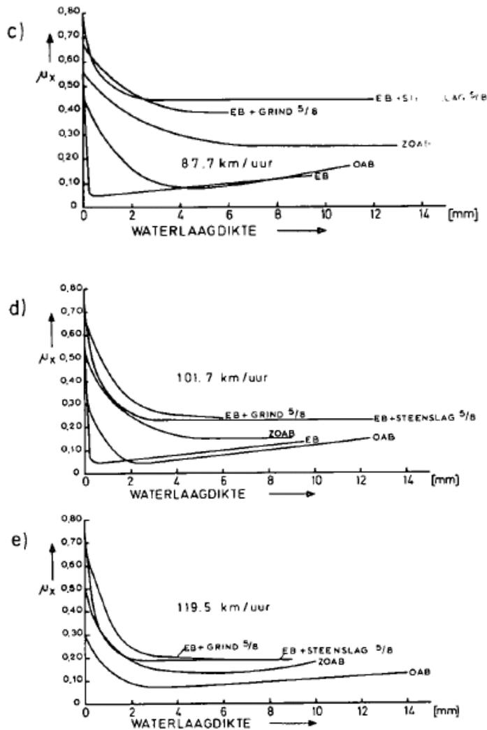
Figure 4 Wet friction coefficient  $\mu_x$  as a function of water layer thickness over pavement asperities (“waterlaagdikte” in Dutch), for five speeds and five surfaces [Welleman 1977].
