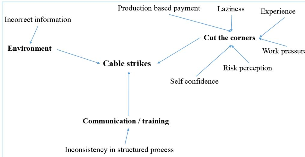
Figure 9, Causal factors of cable strikes
