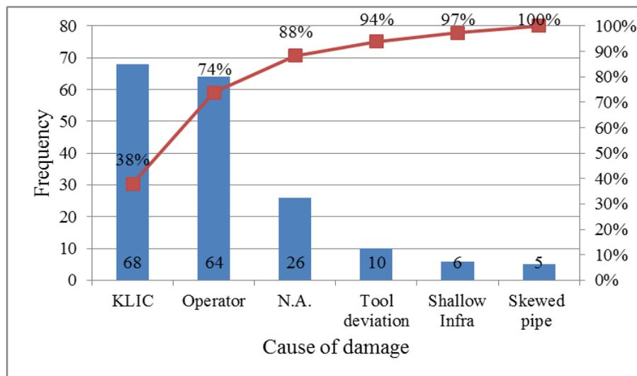
Figure 8, Pareto analysis for causes of damage
