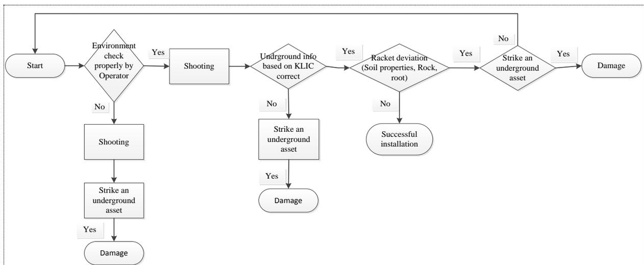
Figure 2, failure demonstration in the boring process
