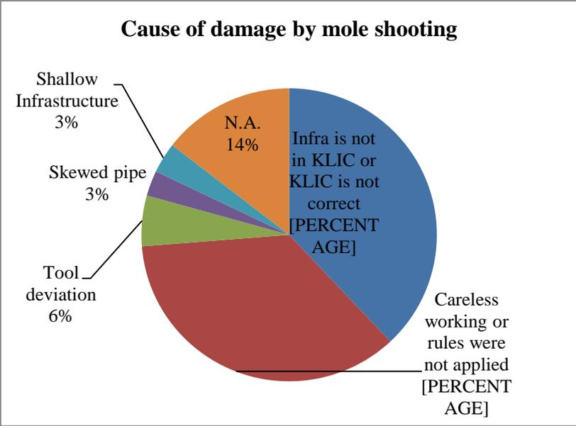
Figure 7, Cause of damage in the gardens by the impact mole
