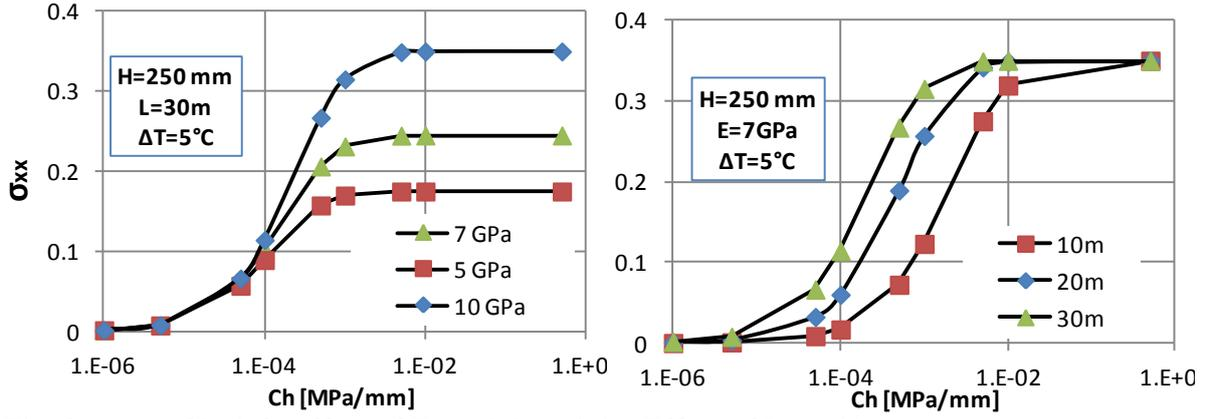
Fig. 2  $\sigma_{xx}$  vs Ch (left: effect of E modulus, right: Effect of Length)
