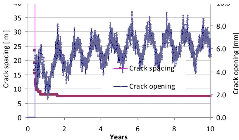
Fig.8 Effects of decreasing the traffic stress on crack spacing and opening
