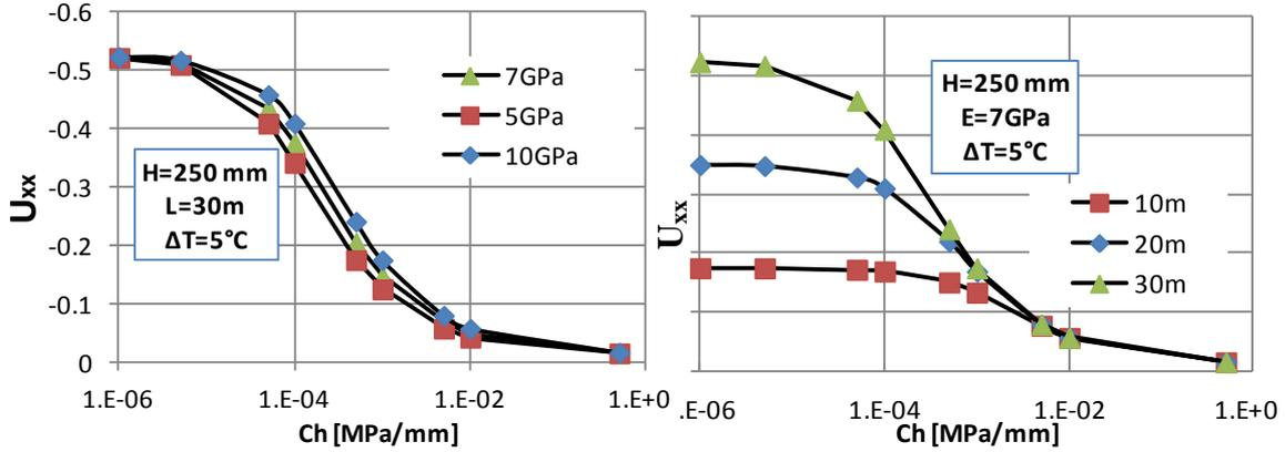
Fig.3  $U_{xx}$  vs Ch (left: effect of E modulus, right: Effect of Length)
