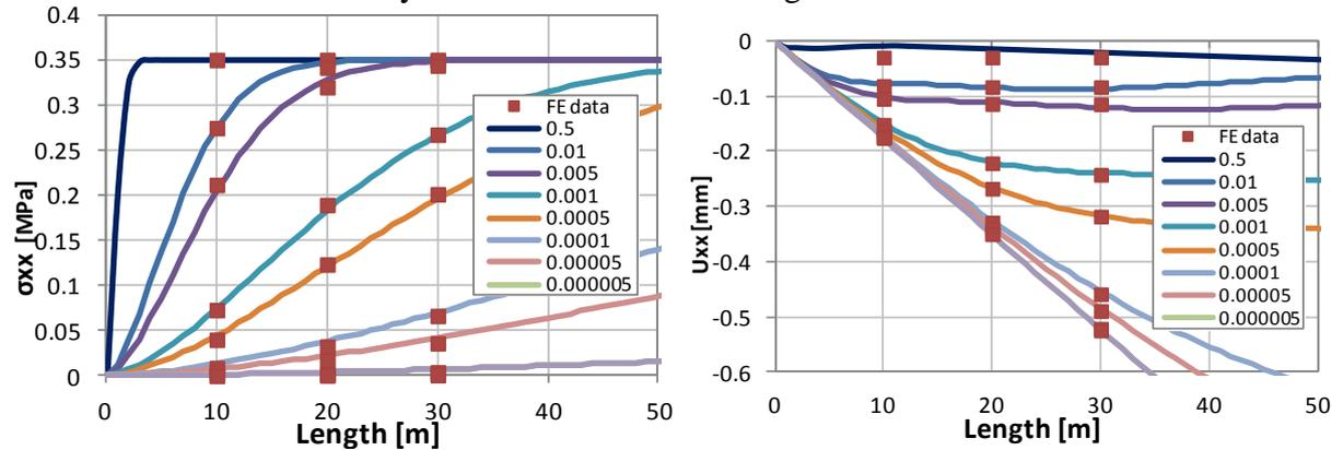
Fig.5 Model and FE simulated data for  $\sigma_{xx}$  and  $U_{xx}$  as a function of slab length and  $Ch$
