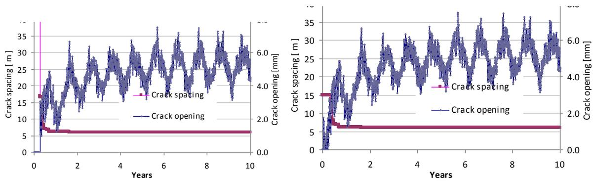
Fig.7 Illustration of model output: crack spacing and opening (left: no pre-cracking, right: pre-cracking at 15m)
