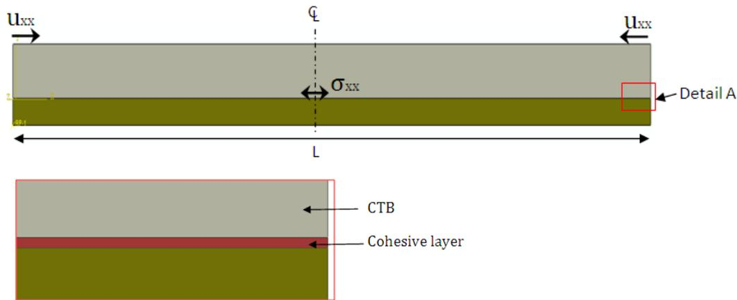
Fig.1 Two dimensional FE Model.
