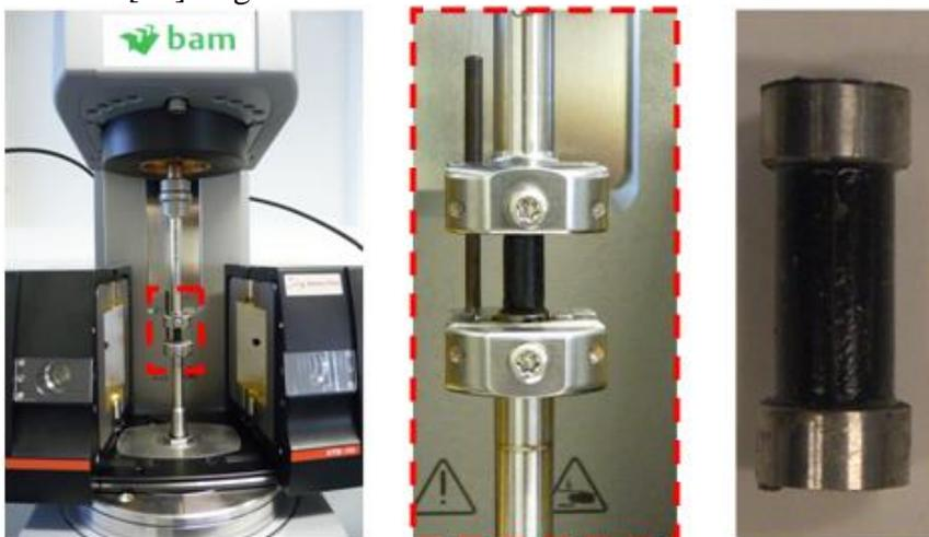
Fig.2 DSR machine(left), detail for mortar test setup(middle), test specimen (right).
