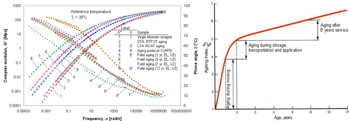
Fig. 1 Effect of field & lab aging on the master curve properties (a)[10], Effect of short and long term aging on bitumen viscosity (b) [11]
