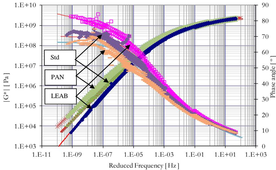
Fig.4 Master curve comparison for standard, LEAB and PAN mortar at Tref= -10°C
