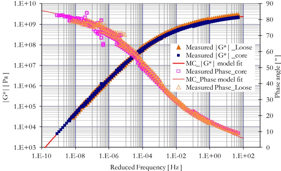
Fig.3 MC comparisons for mortars extracted from loose mix and drilled cores for LEAB
