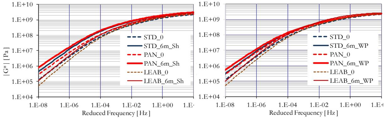
Fig.5. Fresh mortar compared with 6month-old mortar: Mortar taken from shoulder (left), and from the Wheel Path(right).
