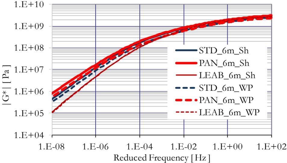
Fig.7 Master curve comparison for mortars taken from pavement shoulder and Wheel path.
