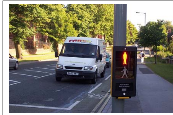
Puffin nearside pedestrian display in foreground with approaching traffic in the background
