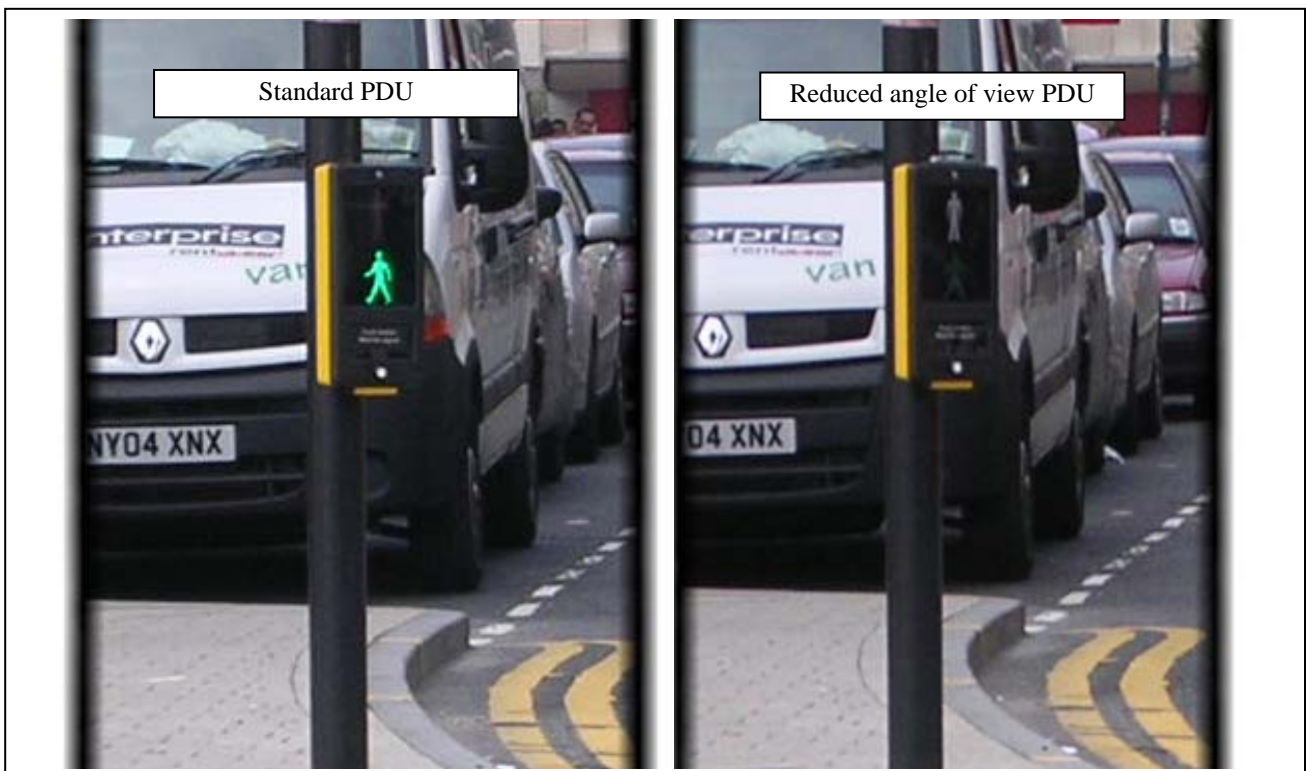
Reduced angle of view PDU (Copyright Sheffield City Council. Reproduced by permission.)
